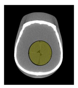
The yellow overlay depicts the location of the insert for this phantom. The imaging insert contains the anatomy while the separate polyethylene dosimetry insert contains the film and TLD.
