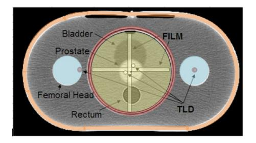
The yellow overlay depicts the location of the insert for this phantom. The imaging insert contains the anatomy while the separate solid HI polystyrene dosimetry insert contains the film and TLD.
